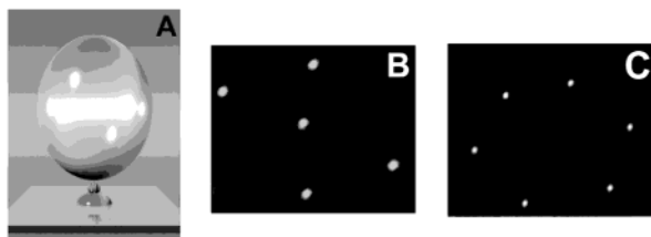
Figure 1. Schematic diagram (A) and CCD photomicrograph (B) of fluorescent microspheres attached to the \gamma subunit of individual F_1 -ATPase molecules immobilized on nickel dot arrays that were created using electron beam lithography.
